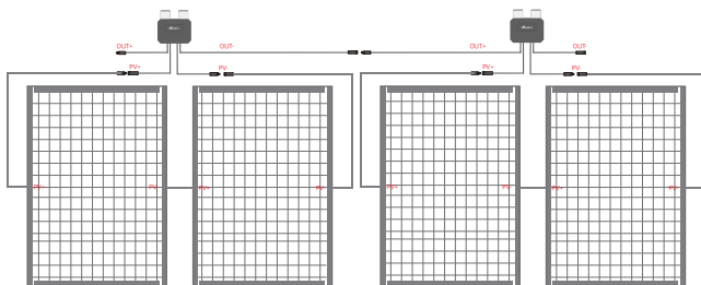
AW-PVRS-A2/B2/C2 1:2 String Parallel Connection Diagram
